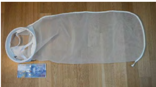
Figure 5.3. A) Nylon filter bag. B) Nylon filter bag in the input of the plastic storage tank.
