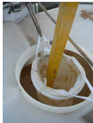
Figure 5.3. A) Nylon filter bag. B) Nylon filter bag in the input of the plastic storage tank.
