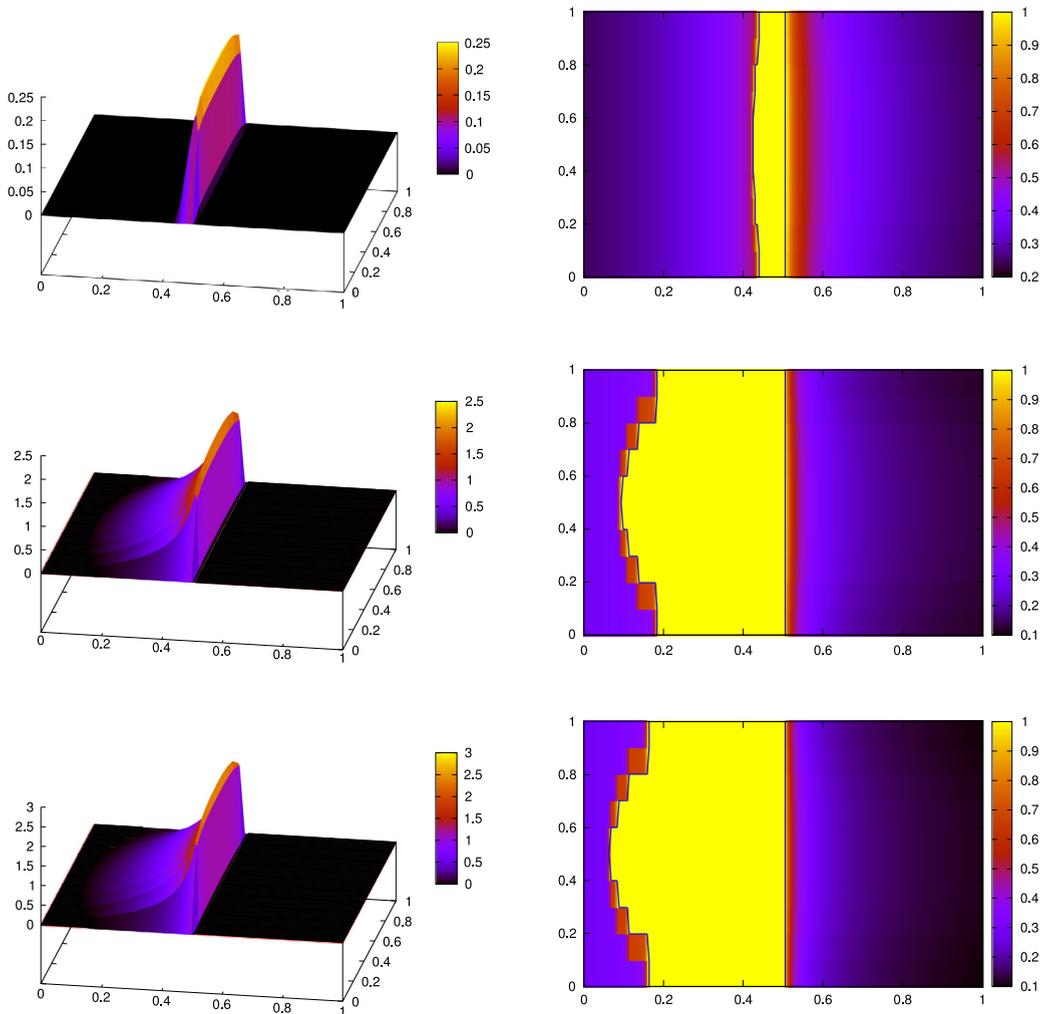
**Fig. 6.** Pressure (left) and corresponding theta-field profiles for different values of  $a$ . Values of  $a$  from top to bottom:  $a = 0.1, 0.01, 0.001$ .
