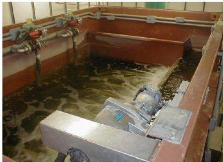
Figura 6: Cloth-Media Filter CMF®, de Aqua-Aerobic Systems
