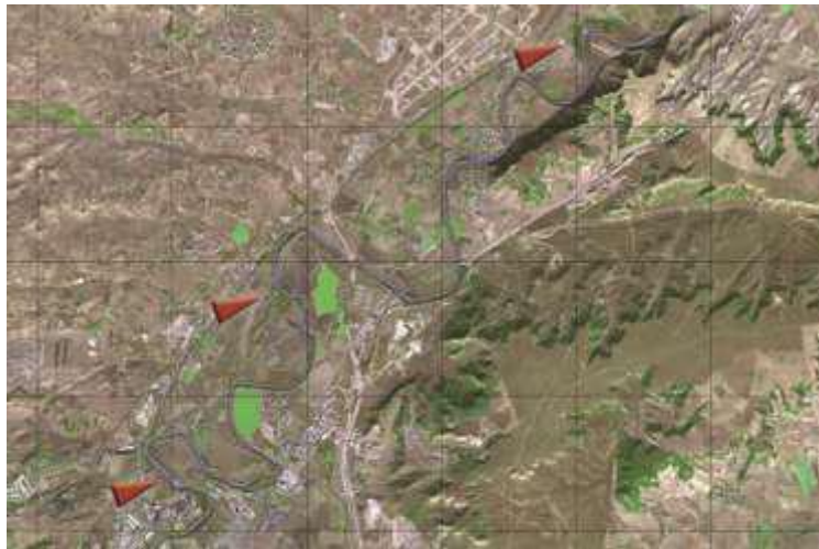
Fig. 5.5. Lower Pisuerga River, upstream Valladolid city. The arrows show the position of three weirs associated to three consecutive SHP. The length of affected stretch is 22.7 km and the medium slope is 0.03 %. The pool-riffle sequence has totally disappeared causing remarkable habitat loss and nutrient retention. As a result, the stretch becomes eutrophic in summer and the ecological regime has shifted from lotic to lentic (Ballarin & Rodriguez, 2013). Source: Iberpix. Instituto Geográfico Nacional, IGN. Grid scale: 2.5 X 2.5 Km.
